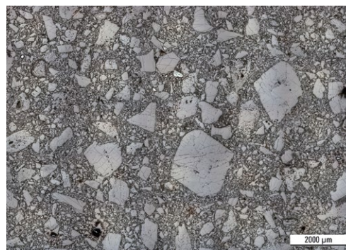
REFRALUSIT® ES matrix Apparent porosity: 18–21%
